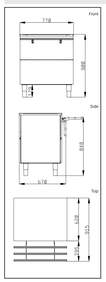
Flexy Compact Ambient Unit on cupboard (2 GN) with one stainless steel tray slider
